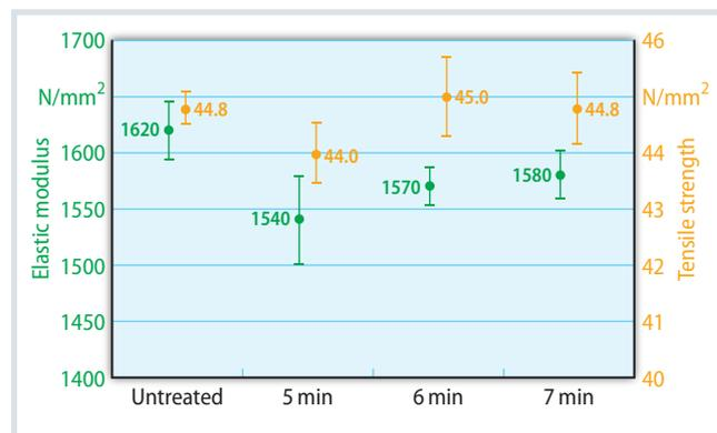
**Fig. 1.** Elastic modulus and tensile strength of PA12
