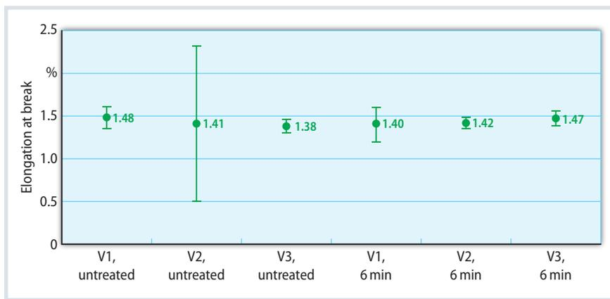
Fig. 4. Elongation at break of glass-filled PA12 Source: University of Duisburg-Essen; graphic: © Hanser
