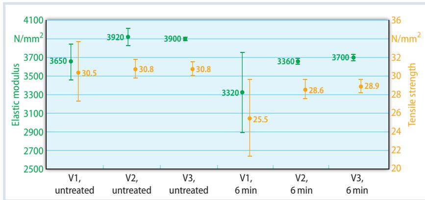
Fig. 3. Elastic modulus and tensile strength of glass-filled PA12 Source: University of Duisburg-Essen; graphic:
